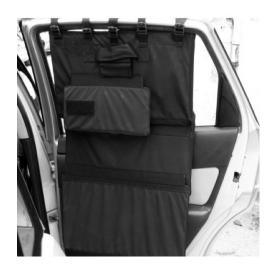
to meet or exceed ballistic resistance as specified within NIJ ceramic plates designed with a 20x30cm view port, to provide Standard 0108.01
