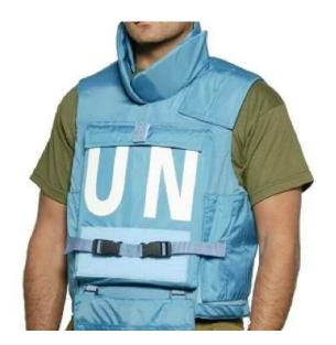
HBA 1103 UN Ballistic Vest is a NIJ STD 0101.06 compliant military vest made from Aramid UD in a heavy duty Nylon carrier. Protection area; front, back, sides, neck and groin.
