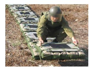
The Mine Mattress prevents the activation of a mine by evenly distributing a person's weight over a large surface, so that the applied weight on the mine located under the mattress is significantly lower than the mine's activation threshold.
